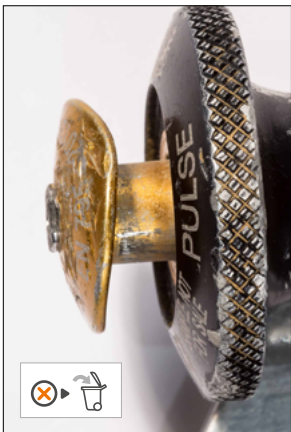
• Marked and deformed plunger
