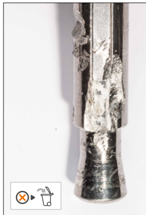
• Marked shaft, broken wedge plate
